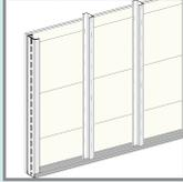
einseitig beplankt<br>planking on one side |
